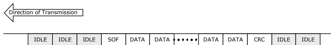
Figure 2-15 General Frame format.
